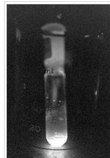
Glow due to the intense radiation from ~300 \mu\text{g} of ^{253}\text{Es} . [25]
