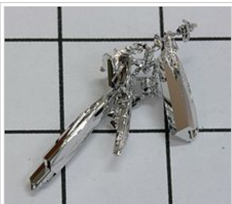
Gas phase grown crystals of ruthenium metal.
